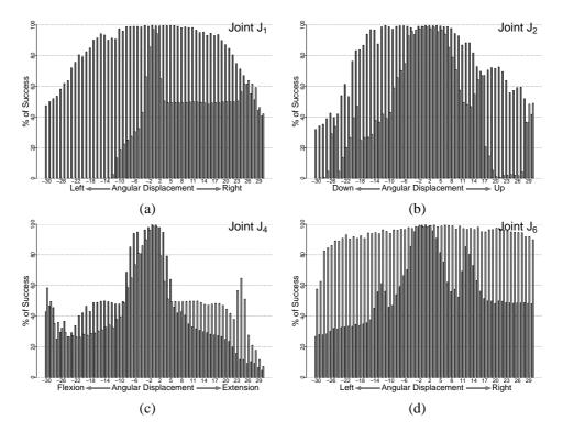
Figure 5: These graphs show the percentage of success in post-evaluation tests in which the initial position of one joint is displaced. Dark grey bars refer to % of success (over 1800 trials) with respect to displacements applied to joints in position A. Light grey bars refer to % of success (over 1800 trials) with respect to displacements applied to joints in position B.
